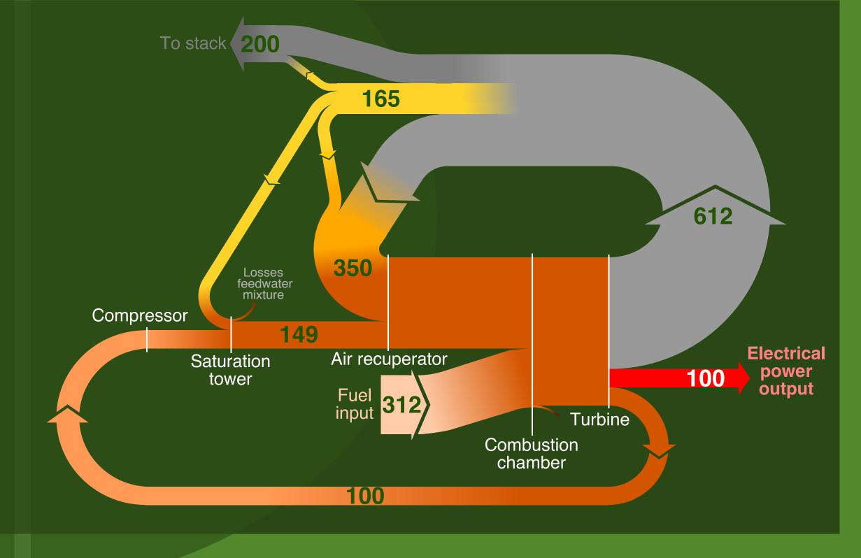
Sankey diagram based on simulations of the Turbec T100 working as an mHAT. The diagram displays the enthalpy flows (in kW) through the different cycle components
